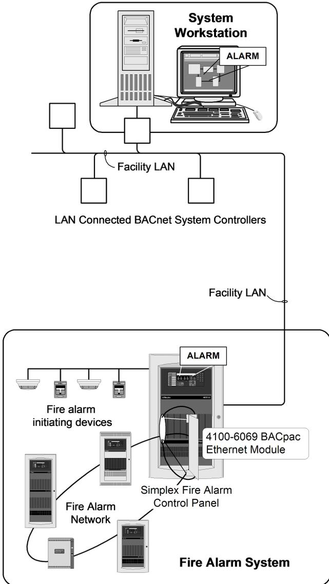
**Figure 1: Typical Building Automation LAN with Simplex Fire Alarm Control Panel and BACpac Portal (shown with 4100ES panel for reference)**
